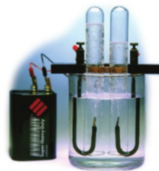
Figure 3 Water decomposes to hydrogen and oxygen gases in a 2:1 volume ratio.
