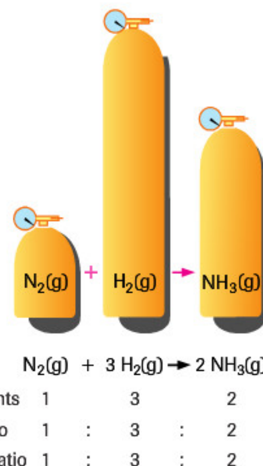
Figure 4 One volume of nitrogen reacts with three volumes of hydrogen, producing two volumes of ammonia.
